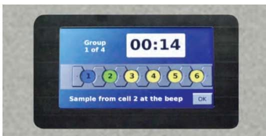
System reminds analyst of sampling time points with visual and audible alerts.
