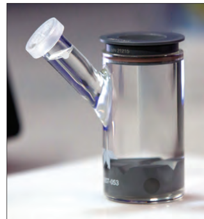
Meniscus through center of fill mark conveniently indicates receptor media has reached the level of the membrane.
