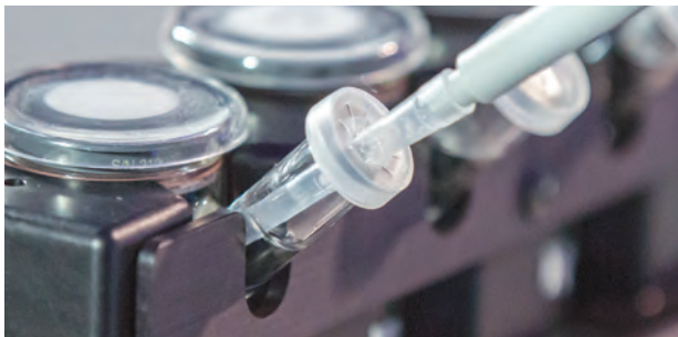
Slotted caps prevent loss of media while allowing manual sampling by pipette or autosampling by probe.
